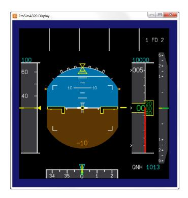
In display setup mode screen elements can be added or removed, they can be moved by dragging with the mouse, the size is adjusted by using the mouse scroll wheel or numeric + and - keys. Remove a displayed element by right clicking and selecting the 'remove ....(name of the display)'. Adding a display element is done by select right mouse click > displays.
